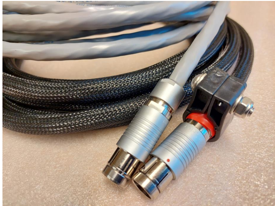
Figure 1: Fischer cables with option 2: individual pair shields (gray) and option 3: all possible shields (black)..
