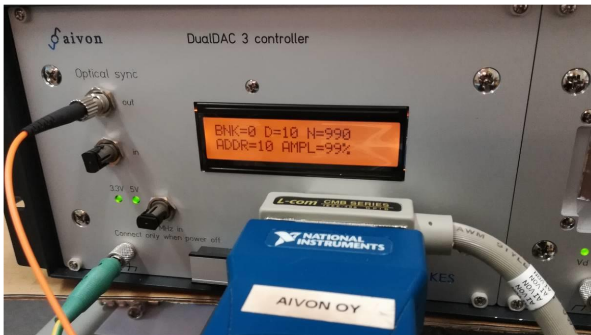
Figure 1: Controller unit with optical sync input/output, 10 MHz clock input (optical) and GPIB connector.
