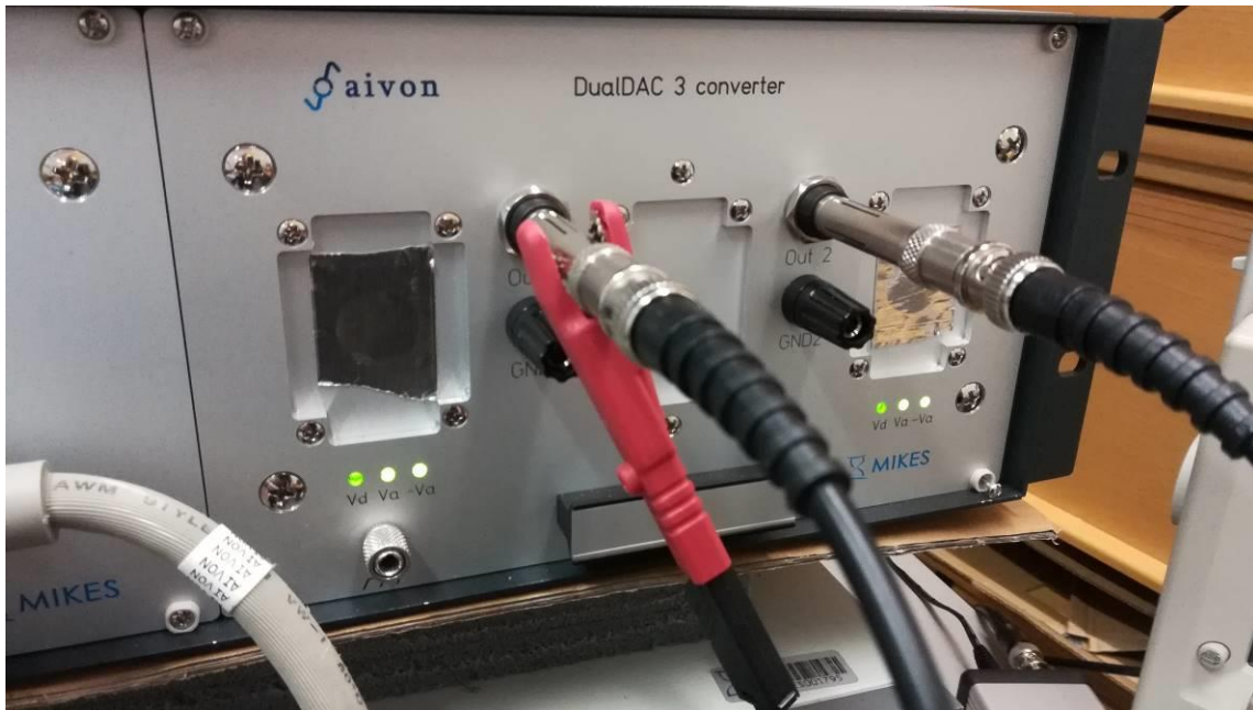
Figure 2: Converter unit with both outputs (BPO connector) connected. Shield is grounded using large crocodile clip.
