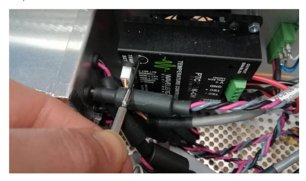
Turn the trimmer and monitor multimeter reading until the desired setpoint is achieved. To obtain more space you can open the rear panel collar screws (6 pcs) and pull the rear panel further away from the main unit.
