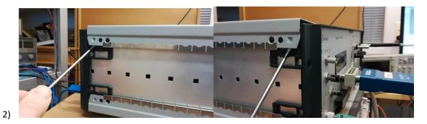
Detach the top panel using a flat screwdriver. There are suitable spots at both ends of the side part of the top panel as shown is the image.
