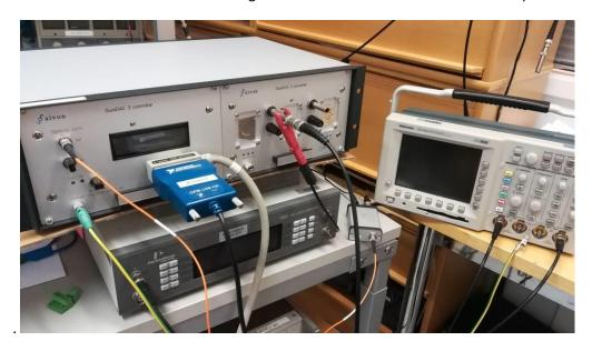
b. Power up the optical-to-TTL converter a.k.a. fibre receiver using the ac/dc wall adapter (12V / 0.5A) delivered with the unit. Green led should indicate operation. Connect optical fibre between fibre receiver and sync out connector of controller unit.
