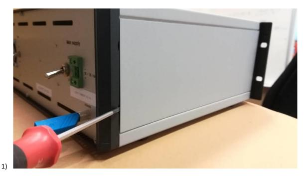
Turn off all power supplies and detach the side panels using a flat screwdriver
