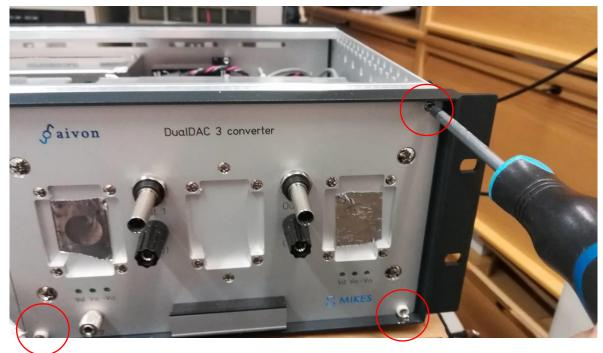
If converter unit or its maintenance lid needs to be removed, undo the four screws at the front corners of the unit.
