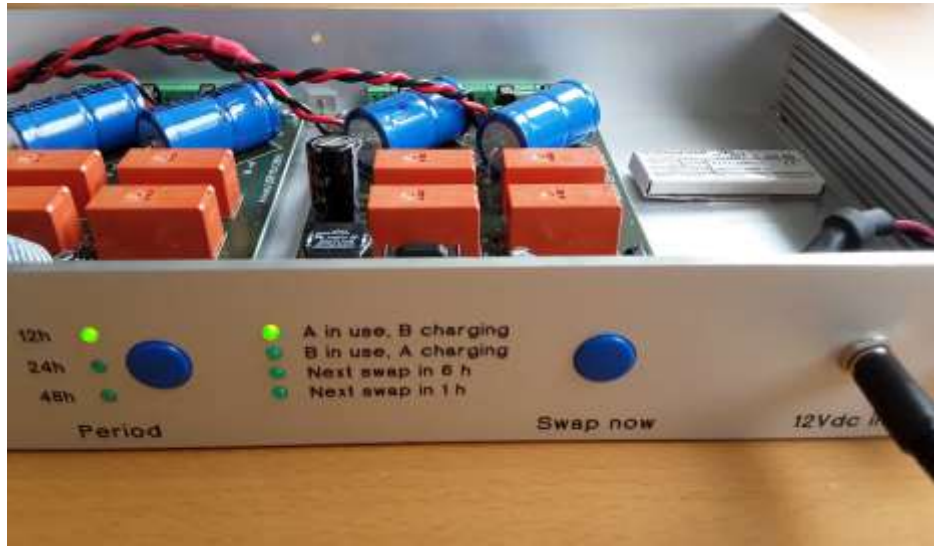
Figure 2: Button switches for swap period, manual swap and power input connector for ac/dc adapter.
