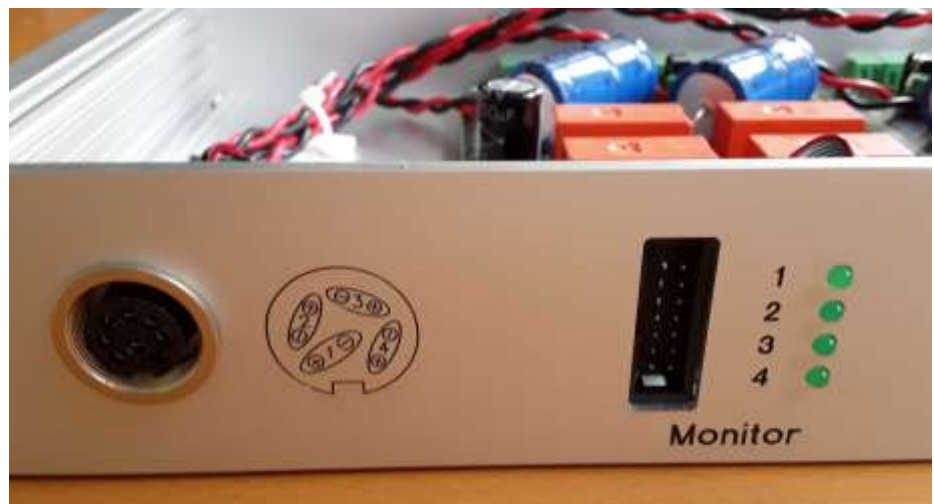
Figure 4: Battery output and monitor connectors. Each battery pair has output pins in circular Binder connector and 2.54 mm pin header (every other row).
