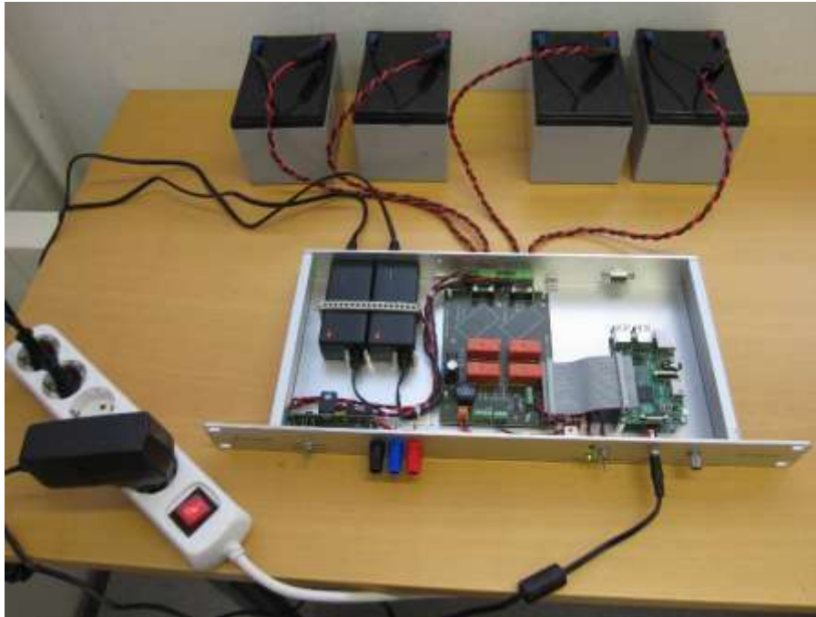
Figure 7: Typical setup with four batteries (i.e. two battery pairs)
