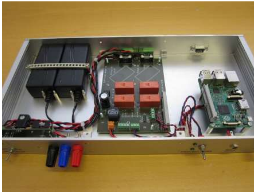
Figure 1: Upper left corner: two battery chargers. Lower left corner: Linear voltage regulator unit attached in front panel. Center: Main relay board. Storage capacitors removed for clarity. Right: Raspberry Pi computer. Upper right corner: spare connector (D9) for user wirings.
