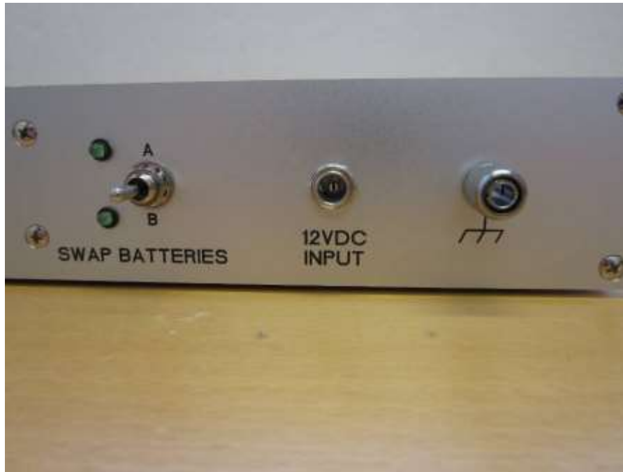
Figure 2: Toggle switch for manual control and power input connector for ac/dc adapter.
