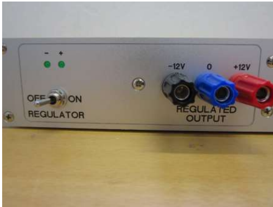
Figure 5: Voltage regulator connectors in front panel. Leds indicate the availability of sufficient battery voltage.
