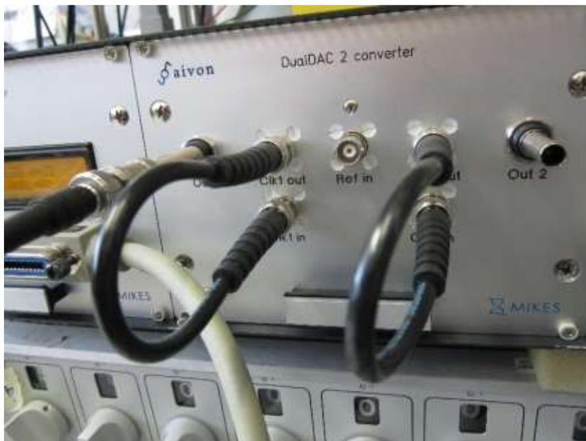
Figure 3: Converter unit with output 1 (BPO connector) connected. Clock in/out connectors shorted with short BNC cables.
