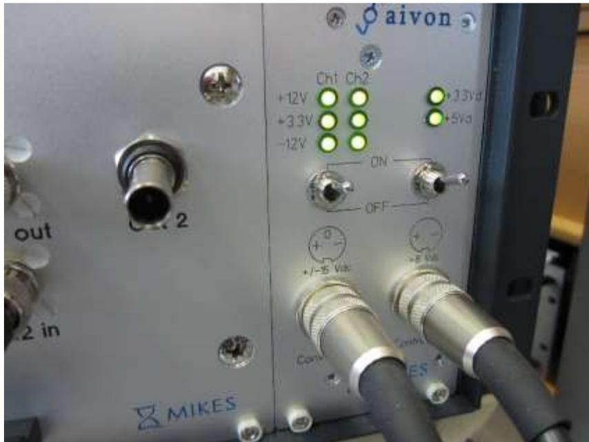
Figure 2: Regulator unit with two Binder-680 connectors as inputs. Power cables from Binder-680 to 4 mm bananas are provided.
