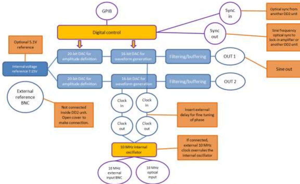
DualDAC 2—system consists of three units attached into 19-inch sub-rack. Converter unit consists of digital-to-analog converters, output driving and filtering circuits and output connectors. Controller unit is composed of digital control circuits for converters and connection to computer. Regulator unit contains voltage regulators for other units. Converter unit is temperature-controlled.
