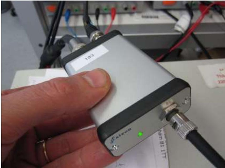
Figure 4: Optical-to-TTL converter a.k.a. fibre receiver
