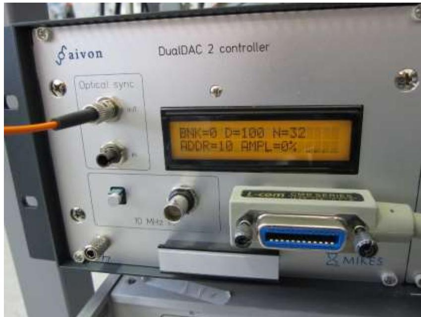
Figure 1: Controller unit with optical sync input/output, 10 MHz clock input (optical/electrical) and GPIB connector.
