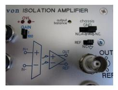
• Model ISO-1D: Output grounding slide switch selects between differential or ground-referenced output modes.
